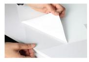
5)Peel off the unwanted color layer part when finish cutting.
