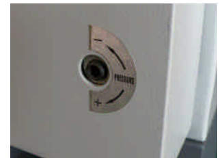
Adjustment for pressure of edge folder
