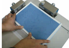
7.push the spine edge firmly onto the exposed adhesive strip
