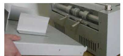
Inserting type of Delivery section
