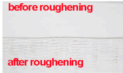
The comparison between before and after roughening
